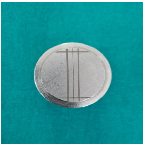
Figure 5: Stainless steel die with 3 vertical lines (X,Y,Z) and 2 horizontal lines. Intersection of cross lines Q and Q' served as beginning and end points of line used for measurement of dimensional accuracy.
