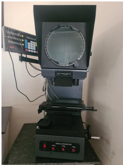
Figure 8: Profile Projector (Radical RPP-3000)
