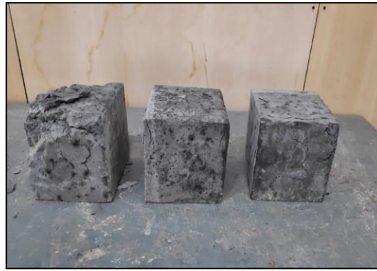
Fig 3: Concrete cubes after testing
